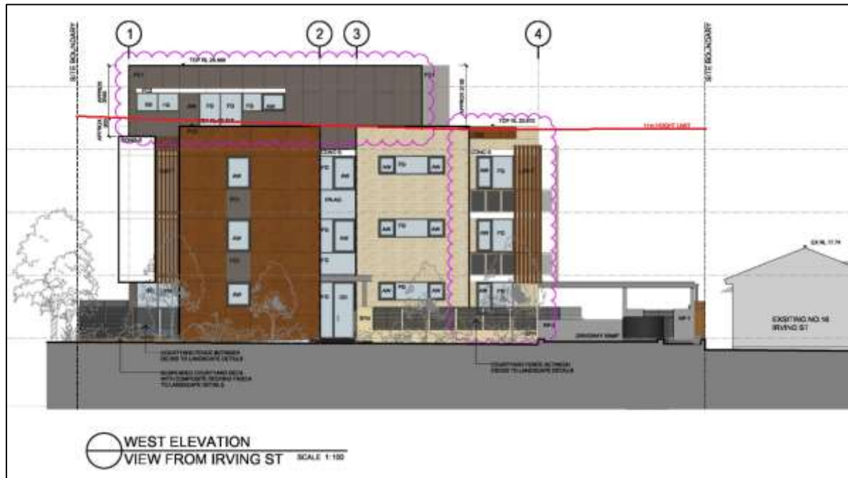
Figure 17: Extract of Western, front elevation showing areas of non-compliance
